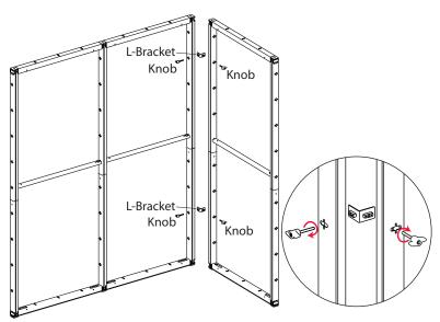
6. To form a corner, attach two L-brackets with knobs. Note: Constructing a room requires a different L-bracket. See the room assembly instructions for details.
