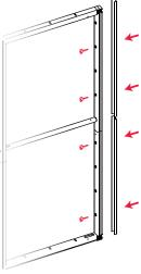
1. To cover the slots at the end of a frame, attach cover profiles with knobs as seen above.
