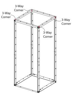
3. Build the upper half of the closet the same way with top vertical bars with3-way corners and four horizontal bars.
