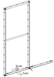
4. Where shown in the kit frame diagram, attach feet to the bottom of the frame with a knob.
