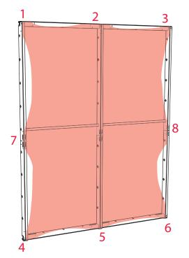
2. Starting in the top/left corner, tuck the graphic. Tuck periodically across the top and then the top/right corner. Repeat for the bottom edge. Tuck the center of the veritical edges.
