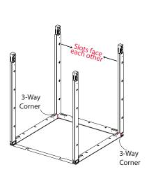
2. Attach two more vertical bars with 3-way corners. Attach one more horizontal bar.
