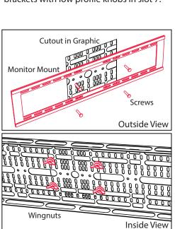
3. Install the fabric graphic with monitor mount cutout aligned over the monitor mount plate. See graphic installation instructions for details.
