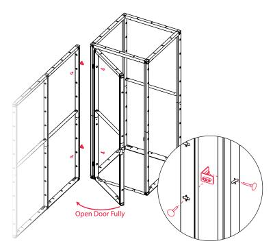
11. To build a wall connected to the room, use two room L-brackets and low-profile knobs. The door must be fully open to attach low-profile knobs.
