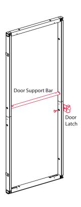
8. Attach the door support bar in the slot above the seam in the vertical bars.
