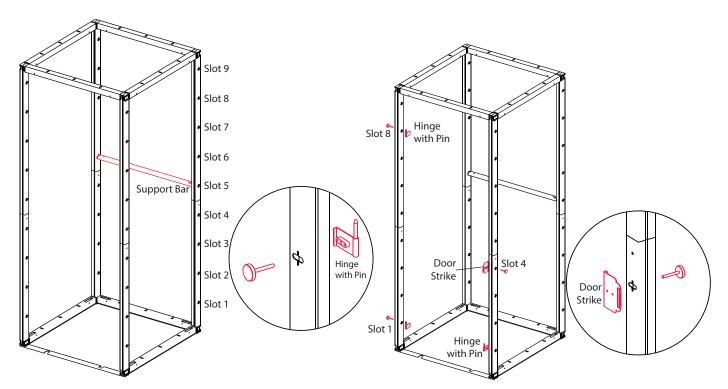
4. Attach a spring-loaded support bar to the wall opposite the door in slot 5.
