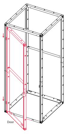
10. Hang the door on the hinges. It is easiest to slide door on hinges when you position door vertical parallel to the storage vertical.
