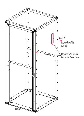
1. Attach two room monitor mount brackets with low profile knobs in slot 7.
