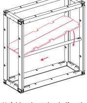
6. Unfold and rest the shelf on the support bars.
