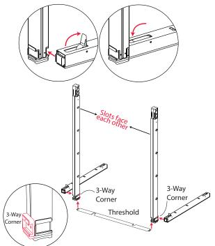
1. Locate two vertical bars with 3-way corners. Attach a horizontal to each of the 3-way corners. Attach the threshold to the bottom of the two verticals.
