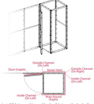
12. Install fabric graphics and backer fabric on the back of the closet. See graphic installation instructions for details.
